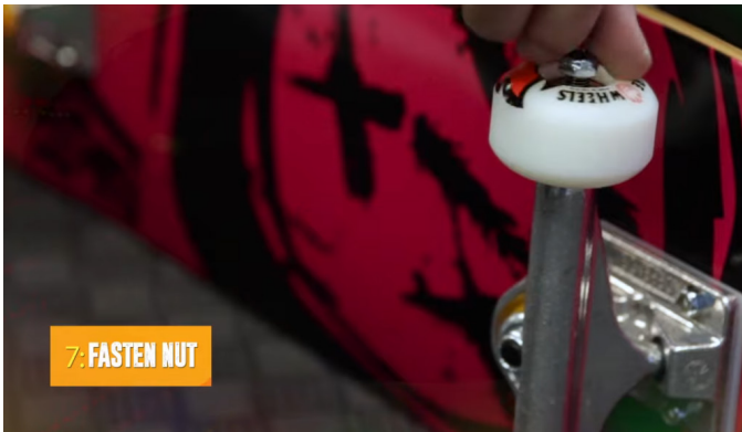
Step 7: With your skate tool or wrench, fasten the nut until there is no play—the wheel should be able to spin freely.
