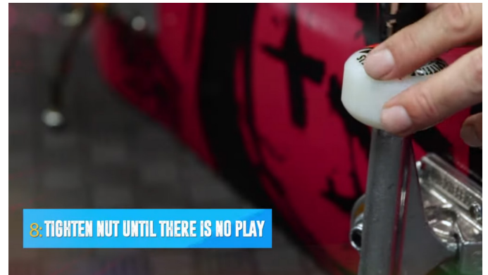
Step 7: With your skate tool or wrench, fasten the nut until there is no play—the wheel should be able to spin freely.
